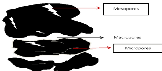
Fig. 3. Schematic model of activated carbon 30
