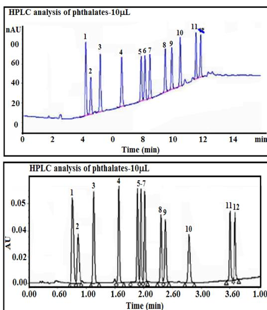
Fig. 5. Comparison of HPLC and UPLC analysis of 12 phthalates
