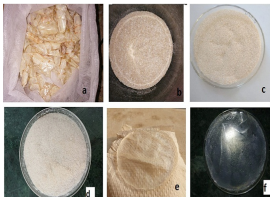
Fig.1. (a) Raw shrimp, (b) Demineralization, (c) Deproteinization, (d) Deacetylation (e) Chitosan Film (f) Chitosan: ZnO biofilm
