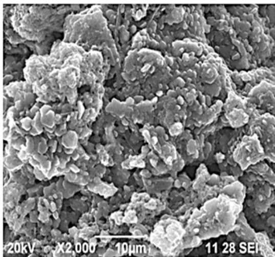
Fig. 4. SEM image of graphene oxide
